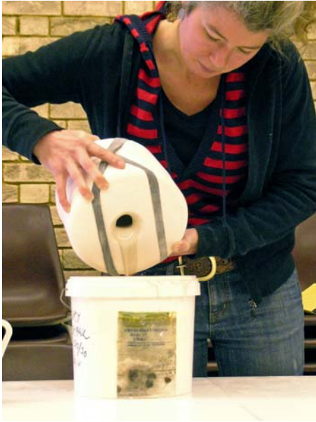
Amy pouring excess slip out of a typical 'globe' mould.
