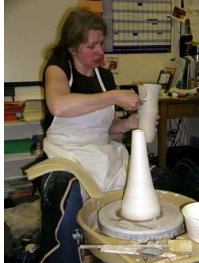
Left: Cutting the rim of a thrown pot before tearing.
