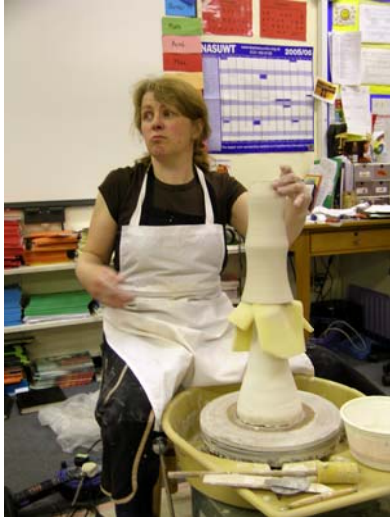
Right: The bases of Pam's pots are turned over a chuck.
