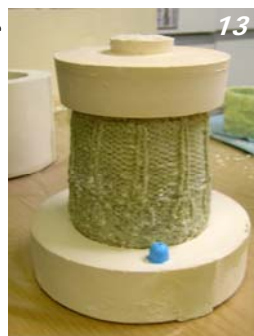
Pic 16: Shrinkage after firing is approximately 20%.
